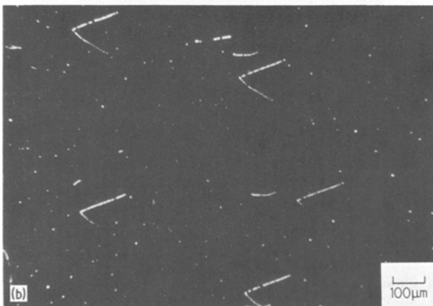
Figure 5 Transmission light micrographs showing (a) runs and (b) "V"s of pinholes in commercially reeled film.
